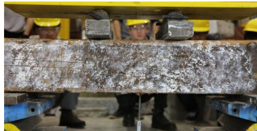
Figure 3. Test set up showing a 4 point bending test
