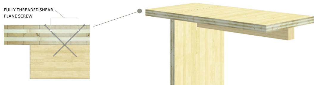
FIGURE 5: CLT PANEL TO BEAM CONNECTION WITH INCLINED SCREWS
