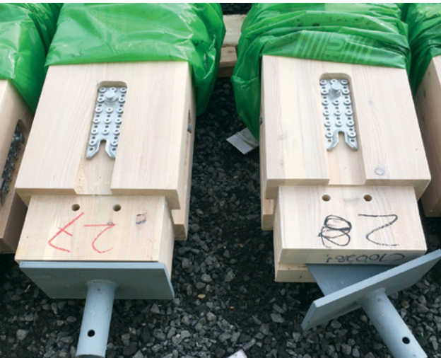
Concealed pre-engineered beam to column connectors
