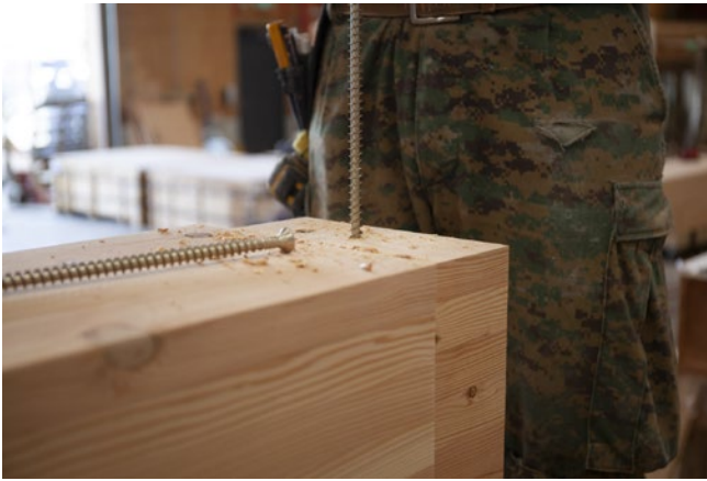
Figure 1. Reinforcement screws being installed in the shop Photo Credit Agency Media, courtesy of naturallywood.com
