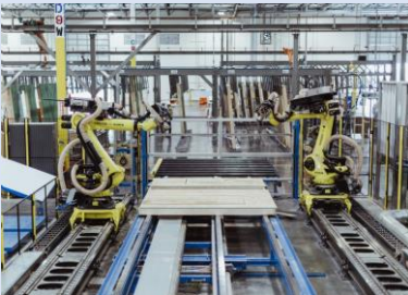
Automated CLT production
