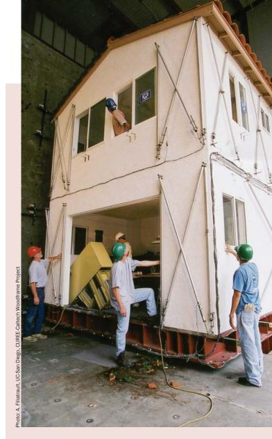
Full-scale shake tests involved the construction of a house on a special platform capable of simulating earthquake loads of different magnitudes.
