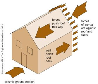
Figure 3: Seismic Forces on a Building
