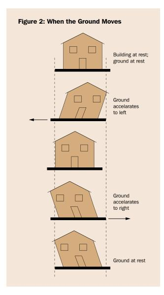
The type of seismic ground motion at a building site is dependant on a number of factors:
